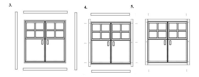
Then insert door frame in to its space from the outside of the structure and attach the rest of the support trims from inside the structure.
