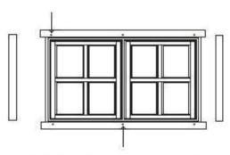
Drill the holes in the support trims and screw them in to the window frame.
