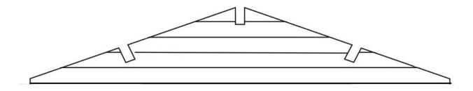
**4.6. Rafters**: The rafters must be mounted horizontally and inserted in the mounting-spaces found on the roof frame triangles.
