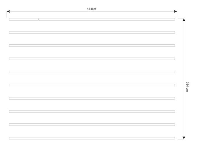
**4.4. Assembling the walls**: place the wall-boards on the bearers as shown below:
