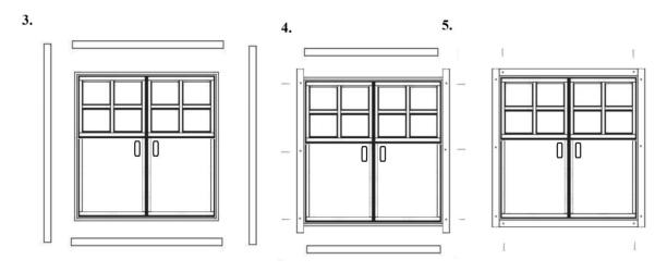
Then insert door frame in to its space from the outside of the structure and attach the rest of the support trims from inside the structure.
