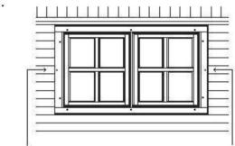
Just insert the window frame in to the space (no screwing)
