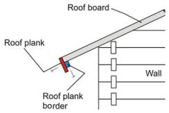
**4.8. Wind-boards:** Place the wind-boards on top of each other to make a 90 degree angle. Now attach these ones on a roof frame triangle and fix with screw in.
