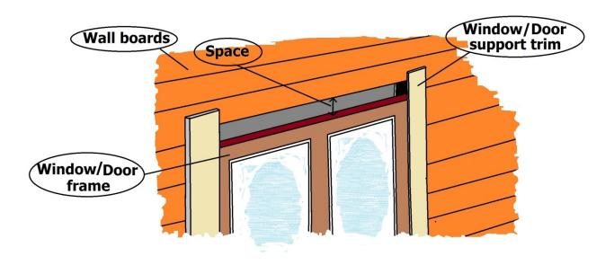
**4.10. Windows:** The windows must be installed in the same way as the doors:
