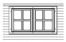
Now screw the rest four support trims in to the window frame from the other side.
