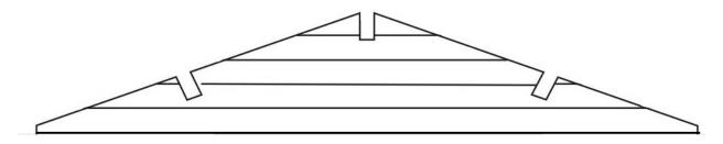
**4.6. Rafters**: The rafters must be mounted horizontally and inserted in the mounting-spaces found on the roof frame triangles.
