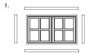
Place the window frame and four support trims on the stable surface.
