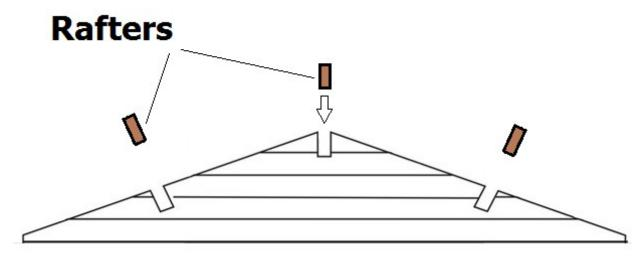
**4.7. Roof-boards:** The next step is to attach the roof-boards vertically and screw them into the rafters. Make sure the ends of the roof-boards are perfectly parallel to each other. Then fix the roof plank boarder under the roof-boards as show below. The roof-plank must be screwed to the roof plank boarder.
