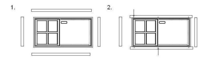
Screw the support trims in to the door frame and insert door frame in to its space from the outside of the structure. Then fix the rest of the support trims from inside the building:
