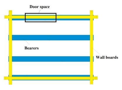
The wall-boards must be placed so that the ends interlock. Now screw the first row of wall-boards into the bearers. All the following rows of placed wall-boards should interlock not only at the ends, but along their length as well. Please screw each new row of wall-boards into the former row to ensure a solid structure.
