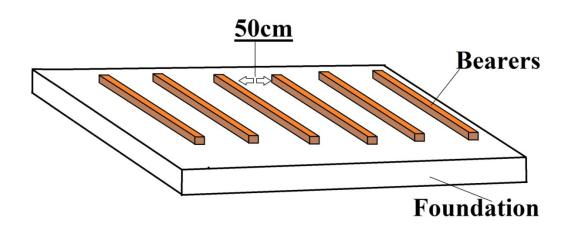
**4.4. Assembling the walls**: place the wall-boards on the bearers as shown below:
