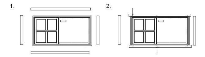
Screw the support trims in to the door frame and insert door frame in to its space from the outside of the structure. Then fix the rest of the support trims from inside the building:
