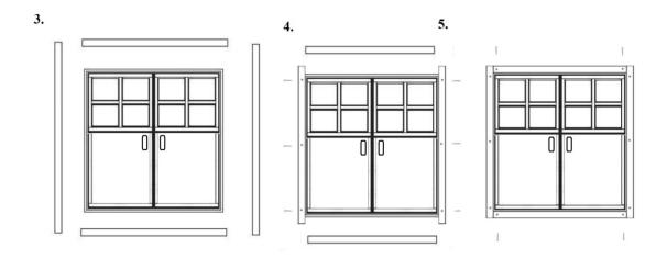
Then insert door frame in to its space from the outside of the structure and attach the rest of the support trims form inside the structure.
