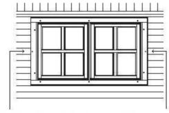
Just insert the window frame in to the space (no screwing)
