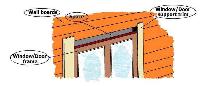
**4.10. Windows:** The windows must be installed in the same way as the door:
