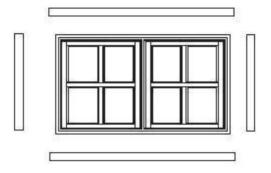
Place the window frame and four support trims on the stable surface.
