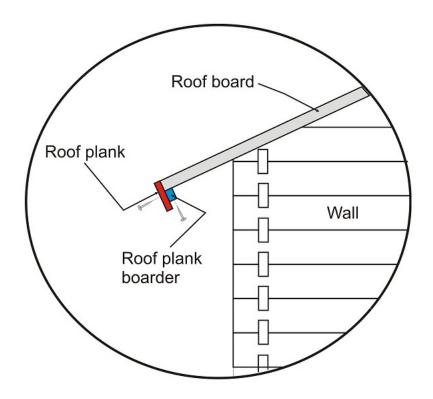
4.8. **Wind-boards:** Place the wind-boards on top of each other to make a 90 degree angle. Now attach these ones on a roof frame triangle and fix with screw in.
