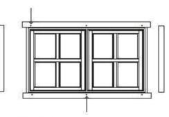
Drill the holes in the support trims and screw them in to the window frame.
